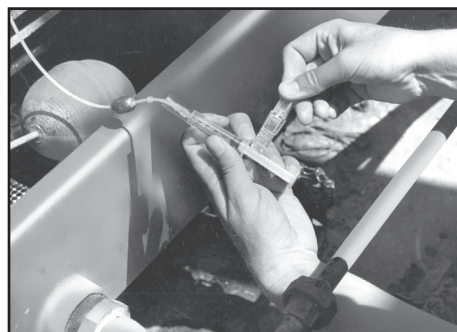
Use syringe to charge Drip Feeder.
