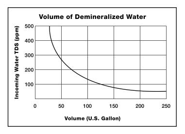
Chart shows capacity of AquaCare T65 cartridge based on incoming water quality. Device has a nominal capacity of 65 gallons at 200 ppm TDS
