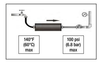
Figure illustrates usage of the cartridge at the jobsite
