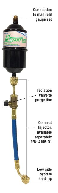
**Note:** Use two A/C ReStart Connect Injects for A/C systems between 5-10 tons. For larger A/C systems, approximately 15% of the oil charge needs to be A/C ReStart. Remove equal amount of existing oil first.
